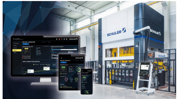
With “Cloud Services”, operating status, pressing force, energy consumption, cooling and lubricating circuits can be monitored. (source: Schuler)
