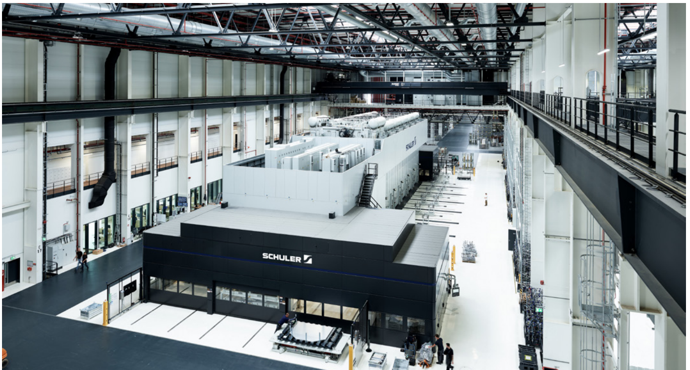
In the Smart Press Shop, Porsche and Schuler operate a servo press line with an output of 20 strokes per minute. (source: Schuler)
